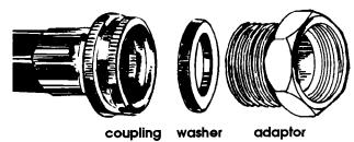
Attach bottom hose with adaptor (inlet marked "H") to hot water faucet. Attach top hose with adaptor (inlet marked "C") to cold water faucet. Tighten couplings to faucet by hand; then use pliers to make final two-thirds turn.
